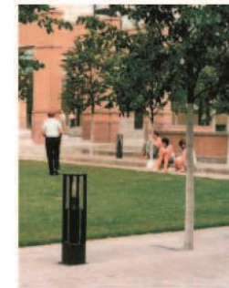
Lighting alternatives; street lighting to define the site area and community, bollard lights to lower the scale to pedestrian, lighting integrated into landscaped areas.
