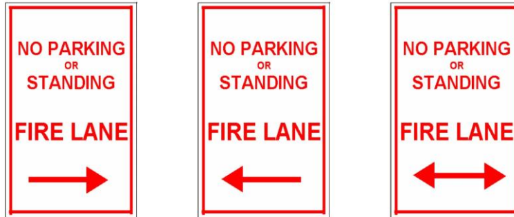
Figure D103.6 Fire lane signs. Delete and substitute as follows.
