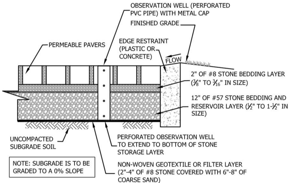
Figure 1. Typical Residential Permeable Paver Detail (N.T.S.)
