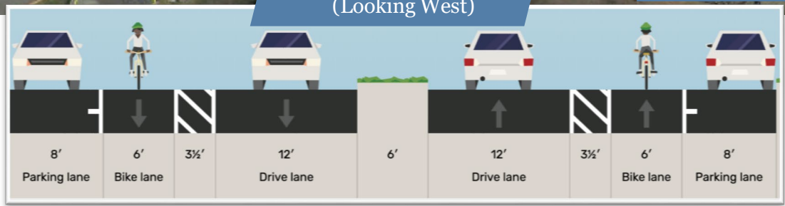
Typical Cross Section (Looking West)
